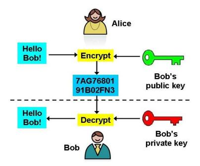
Ciphertext is combined with the **recipients private key** and **decryption** algorithm to produce plain text.
