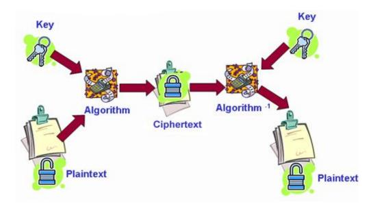
Plain text is combined with the secret key and encryption algorithm to produce ciphertext.
