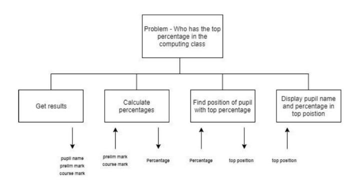
• **Refinements** — break down the design from the top level into smaller steps. They can be shown separately from the top level design or below the top level design.
